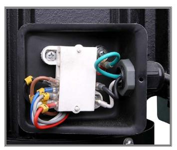
Figure 35. Motor junction box wiring.
